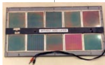
Double junction amorphous silicon solar module fabricated at IACS with 6% stabilised efficiency (without laser scribing)
