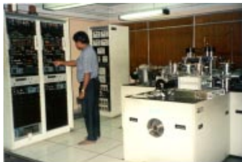
Multichamber PECVD system for fabrication of a-Si thin film solar cell
